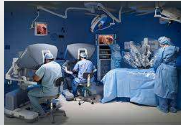
Teleoperated robot-assisted surgical system for minimally invasive procedures. (Credit: Intuitive Surgical, Inc.)
